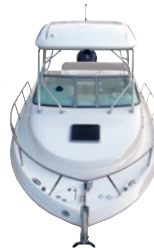
■ Rather than a pulpit, the Robalo R245 handles anchoring duties via a conventional bow roller.
