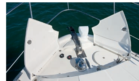
Windlass, fender locker, raw and freshwater outlets under a smart two-hatch set-up.
